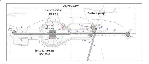
The Pass-by Noise facility at AMTC offers an ISO 10844 certified surface. Track layout and design allows for efficient test setup with cables pre-run underground to pull boxes near the track.
